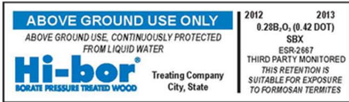
FIGURE 3—TYPICAL HI-BOR® BRAND BORATE PRESSURE TREATED STAMP DESIGN (0.42 DOT)
